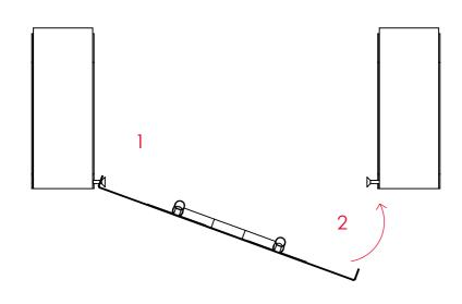
Clip one side of the Heat Cloud panel into the protruding wood screw (1).
