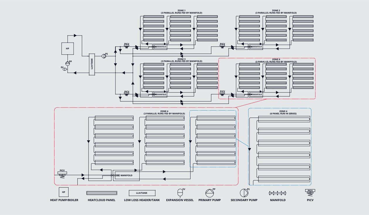
Figure 7. Example of single zone piping
